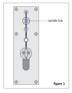
Apply the front and back plates with the neoprene seals in position against the door, over the protruding ends of the spindles.
