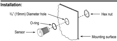
**Note:** To ensure proper operation, make sure no objects sit or come within 11<sup>3</sup>/<sub>4</sub>" (30cm) (60° to the left and right) of the front of the IR proximity sensor to avoid interference.
