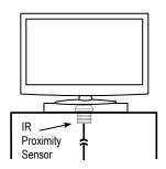
Place the sensor under a painting or other valuable object. If the object is removed from the sensor, the sensor will trigger an alarm to alert the owner that the item is out of place.
