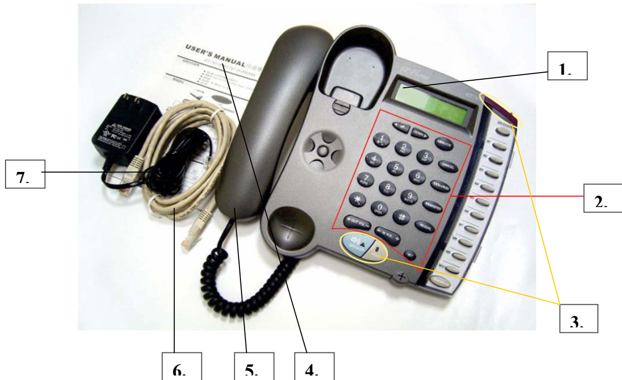
Figure 1. Key parts of the VOIP 2747 series IP Phone
