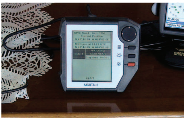
FIGURE 83-3 Crew overboard alarms are capable of alerting the vessel's crew to an emergency, while storing the precise coordinates where the crew member fell overboard.
