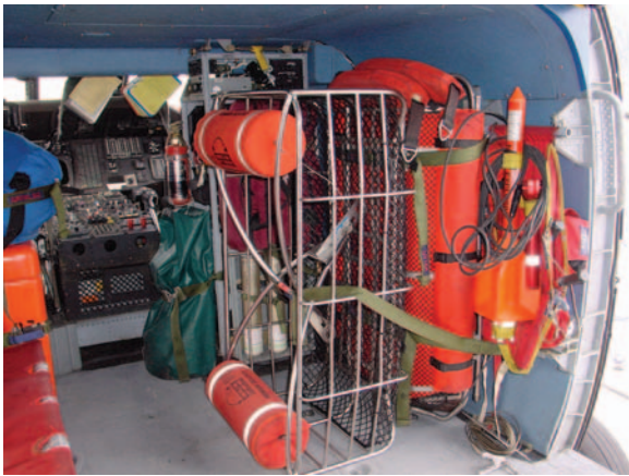
FIGURE 83-18 Coast Guard HH-60 Jayhawk helicopters carry a wide variety of gear to hoist victims and to assist crews in saving their vessels.
