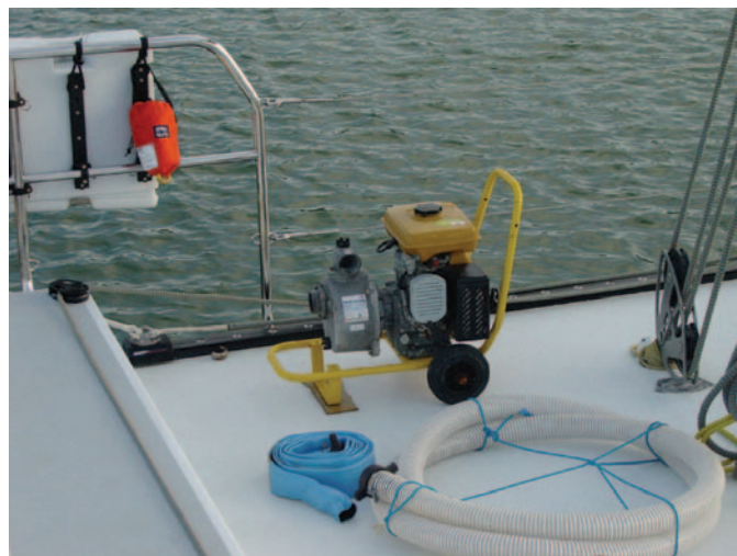
FIGURE 83-8 Large vessels may elect to have substantial emergency pumps onboard, which can keep up with flooding from modest hull breaches. Note also the crew overboard device on the pushpit and the throw rope.
