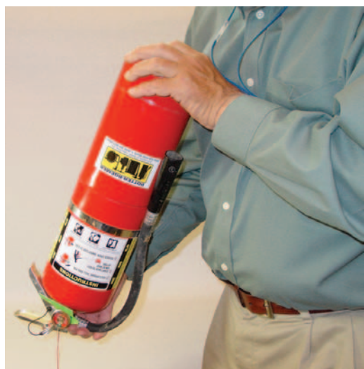
FIGURE 83-10 Dry chemical fire extinguishers should be inspected to ensure the pressure gauge indicates a full charge and should be inverted regularly to unpack the extinguishing agent.
