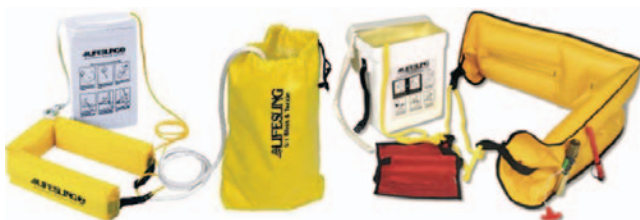
FIGURE 83-6 The Lifesling has become the preferred man overboard recovery system. The flotation horseshoe collar with attached retrieving line can be thrown or towed to the overboard person and used as a lifting sling to hoist the crew member back on board. An inflatable model comes in a throw bag.
