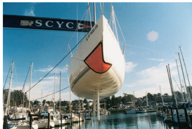
FIGURE 83-9 Triangular patches made from coated fabrics can be held in place with lines attached to each corner.
