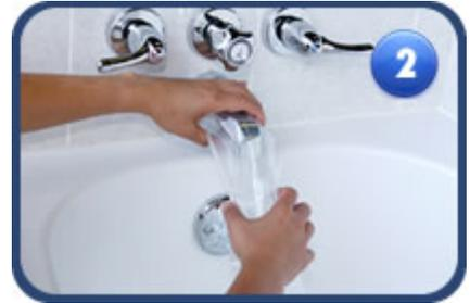
Unscrew the nozzle cap that is closest to the faucet and attach the fill sock to that nozzle by turning it clockwise until tight. Slide the other end of the fill sock over the bathtub faucet.
