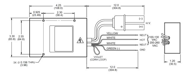
\* When loop is cut, 3-7 second turn-on delay is deactivated
