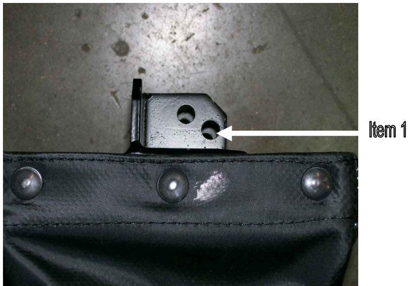
Figure 15. Vinyl Chain Bag Installation Connection
