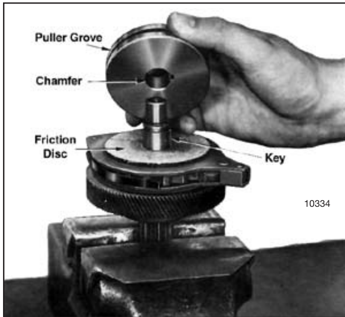
Figure 7-22. View Showing Load Brake Flange Removed
