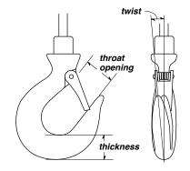
The wire rope assembly must be replaced if the throat opening is 15% wider than nominal, if the thickness is 10% less than nominal, or if the hook is twisted 10° or more.
