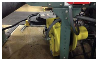
Failing cable due to the “corkscrew” effect
