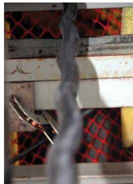
Failing cable due to the “corkscrew” effect
