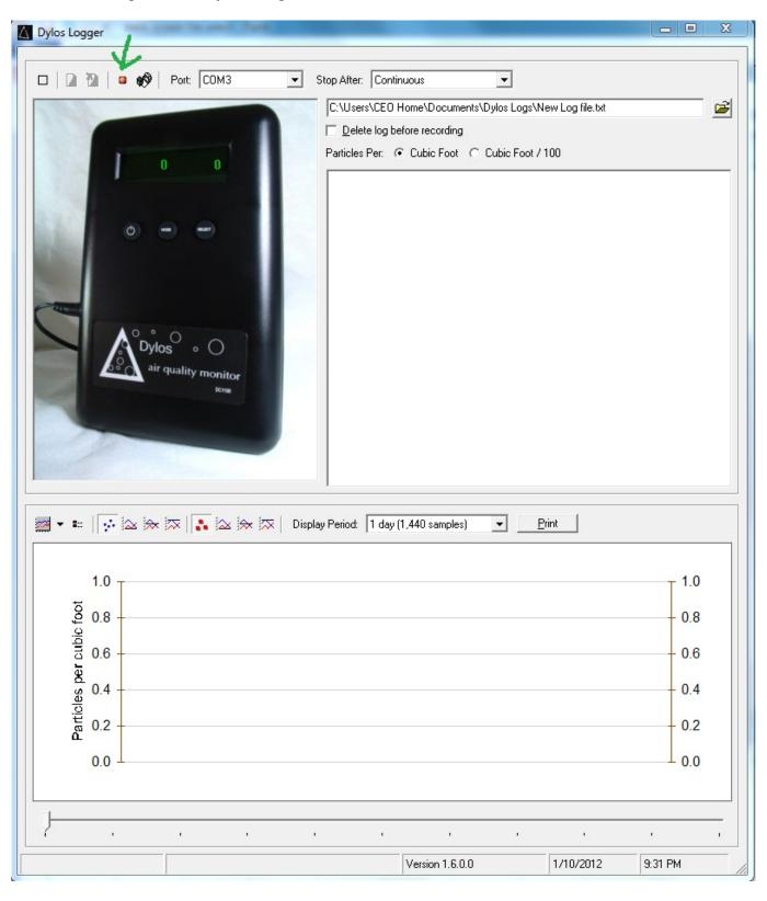
The DC1100 or DC1700 output a reading every minute which represents the average particle concentration over that minute. This data will be stored to the selected log file as well as being displayed in the data window and being graphed in the graph window. The screenshot below shows the DylosLogger after several minutes of data logging:
