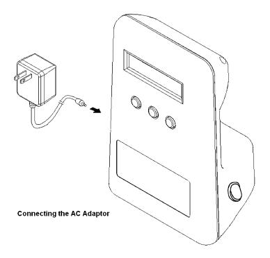
The DC1700-PM also has an internal 7.2V NiMH battery which can provide up to 6 hours of operation. To charge the internal battery, plug the DC1700-PM into AC, but don't turn the unit on. Refer to page 19 for complete instructions. (Note: It may take 12 or more hours to charge a fully discharged battery)
