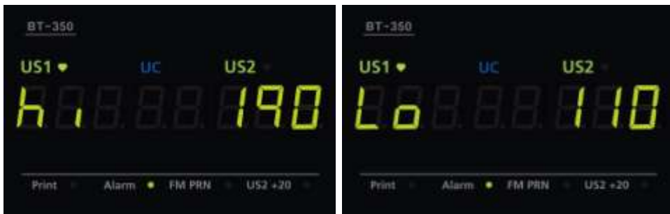
Fig. 4.3 Alarm Upper /Lower Limit
