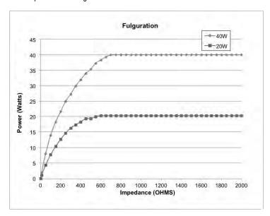
Figure A - 8 Output power vs impedance for Bipolar mode
