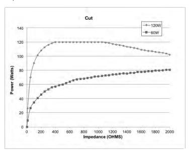
Figure A – 5 Output power vs impedance for Blend mode
