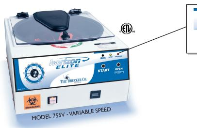
Control panel lights inform the operator of the machine's current status
