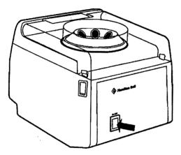
5. 60 MINUTE TIMER OPERATION – Rotate the timer knob on the lower right side of the centrifuge unit in a clockwise direction past the 10 minute mark. Then set the timer to the desired timing interval. The indicator light on the lower left side of the centrifuge unit will become illuminated and the centrifuge will start operating. The centrifugation process will stop when the timer returns to the zero position. See illustration.
