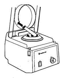
Aluminum shields are easily removable for cleaning.
