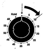
For continuous operation, rotate the timer knob counterclockwise to the HOLD mark. To stop the centrifugation process, rotate the knob clockwise to the 0 (zero) mark. See illustration.
