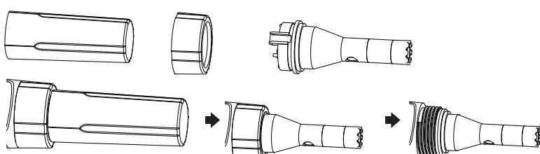
The membrane part is replaceable.
