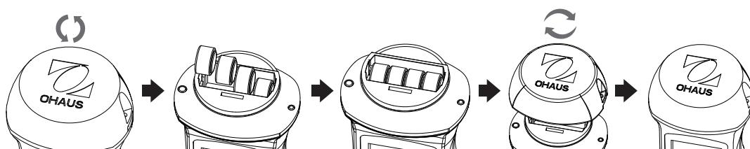
The electrode is replaceable.
