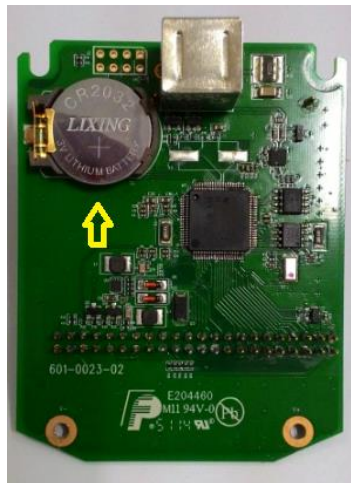
Figure 2-5. Location of the battery at the back of the main PCBA. (Type CR2032)
