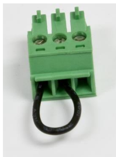
Figure 5-4: Jumper Wire Between COM1 Transmit and Receive Terminals
