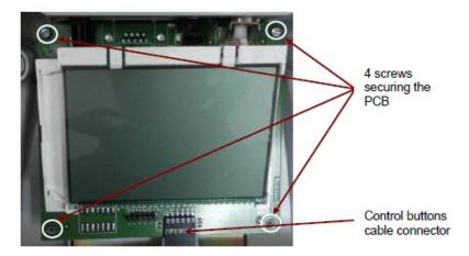
Figure 2-2. Main Printed Circuit Board with display.
