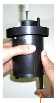
To reset the piston, remove the piston from the housing. Holding the piston, push down on the vertical rod all the way down it may click.
