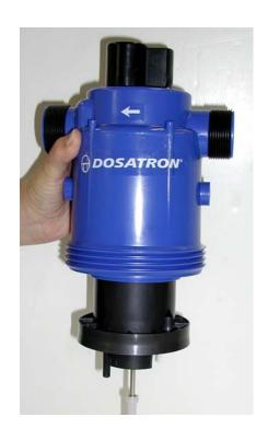
Insert piston into the upper half way up, hold the upper housing of the unit with the piston facing down, then let go of the piston. The piston should be snug in the upper housing and the piston should not fall out, if it does, the piston shell needs to be replaced. Also inspect the inside of the upper housing and look for deep vertical scratches, if this is the case, the upper housing needs to be replaced.
