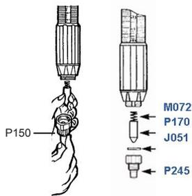
6. Insert new white stem into black sleeve, making sure black key in sleeve is aligned with long groove in stem.
