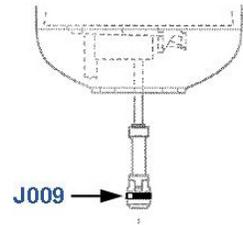
**!** To remove seal easily without tools, squeeze it on either side to raise the seal, then slide it over the groove. Using tools could damage the plunger.
