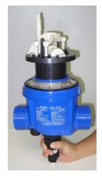
Insert the lower part of the piston half way down the body. Then let go of the piston. The piston should be snug in the body and the piston should not fall in, if it does, the piston shell needs to be replaced. Also inspect the inside of the body and look for deep vertical scratches, if this is the case, the body needs to be replaced.
