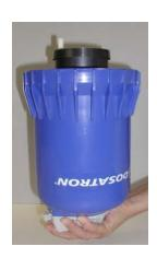
Insert the piston into the upside down bell housing half way down. Then let go of the piston. The piston should be snug in the upper housing and should not fall in. If it does, the piston shell needs to be replaced. Also inspect the inside of the bell housing and look for deep vertical scratches or excessive wear. If this is the case, the bell housing needs to be replaced.
