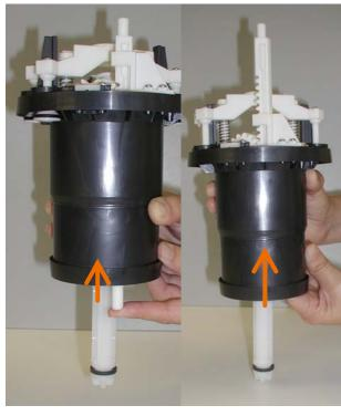
To reset the piston, remove the piston from the dispenser. Holding the piston push down on the vertical rod all the way down, it may click. Push the vertical rod all the way up, it should click. Push the vertical rod all the way down once more and it should click. Insert the piston inside the dispenser.
