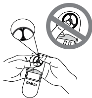
Replacing the Impeller
