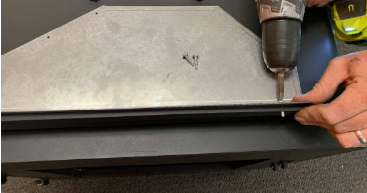
Attach the top front blower duct to the frame with 3 machine screws
